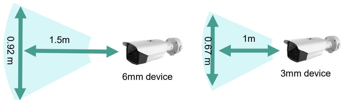
Thermographic fever screening scheme cover range
